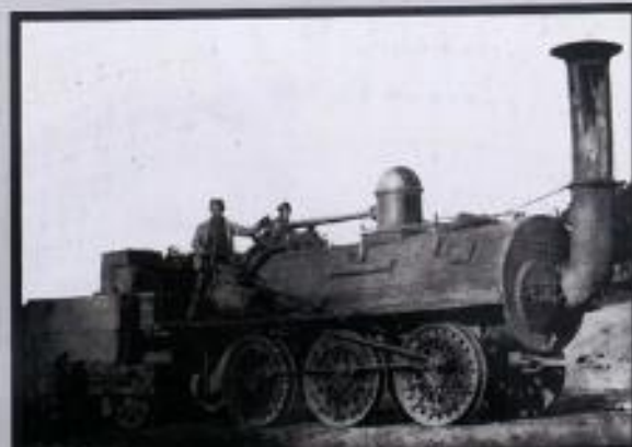
A very early photograph of the type of Stockton & Darlington Railway locomotive that would have been seen crossing the bridge in the mid-19th century. This is locomotive No. 9, unusually named Middesbrough . It was built by the Darlington engineer William Lister in 1839 and worked on the line until 1865.
